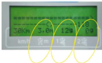
Spreading quantity compartment 1
