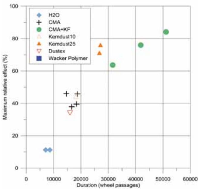
Fig. 22 Comparison of the effect of different dust suppressants
