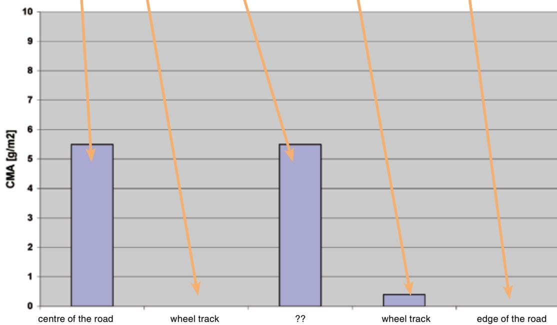
Fig. 26 Test track Rudolfsbahngürtel, cross section measurements (schematic) after 4 hours and 2,000 vehicles, average after 4 h application ( $10 \text{ g/m}^2$  CMA).
