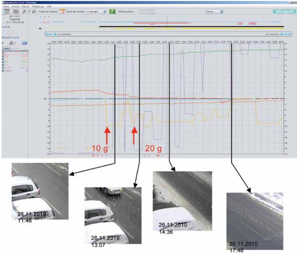
Fig. 25 Boschung's ground sensor online measuring system, test track, comparison of reduced freezing points of 10 g CMA and 20 g NaCl.
