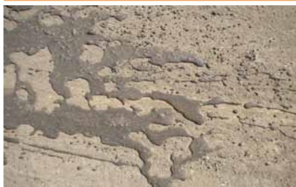
Fig. 8 CMA on a dry dust layer
