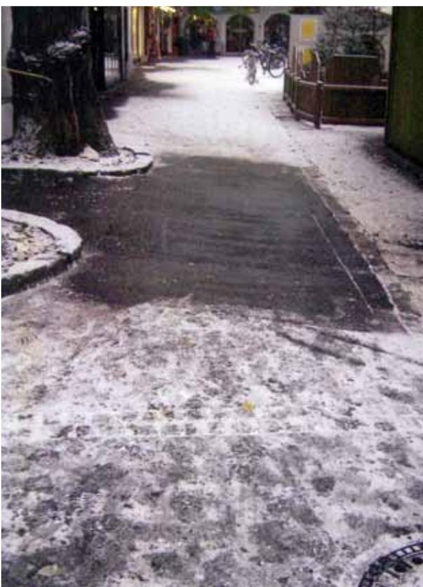
**Fig. 5** Application in the pedestrian area of Lienz: a de-icing effect can be clearly observed up to a new-snow depth of approx. 3 cm.
