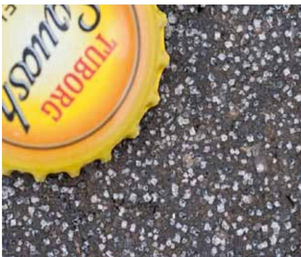
Fig. 4 Salt crystals on road asphalt
