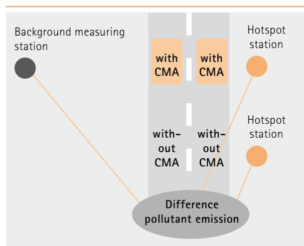
**Fig. 10** Scheme of measuring set-up – air-quality measuring station of Graz University of Technology
