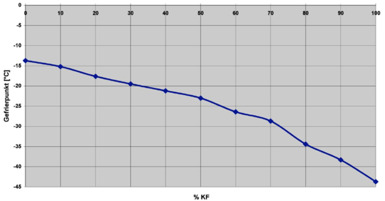
Fig. 31 Freezing point of CMA, CMA:KF mixtures (w/w %) and KF in an aqueous solution; determined as per the ASTM D 1177 method by Saybolt, Denmark, analysis report no. 102/11639-0/11, of 19.9.2011, commissioned by Nordisk Aluminat, DK.
