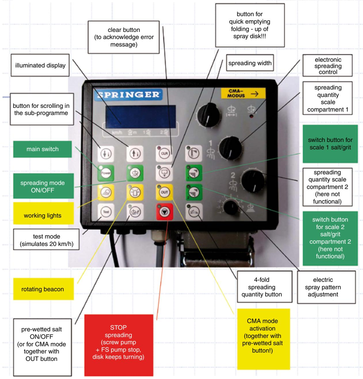
Fig. 23 Control panel, spreading system by the company Springer
